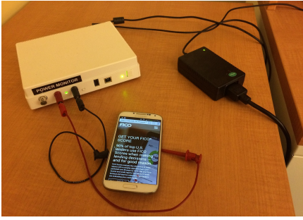
Figure 1: Our hardware setup showing the Samsung S4 under test connected to the Monsoon power monitor.
