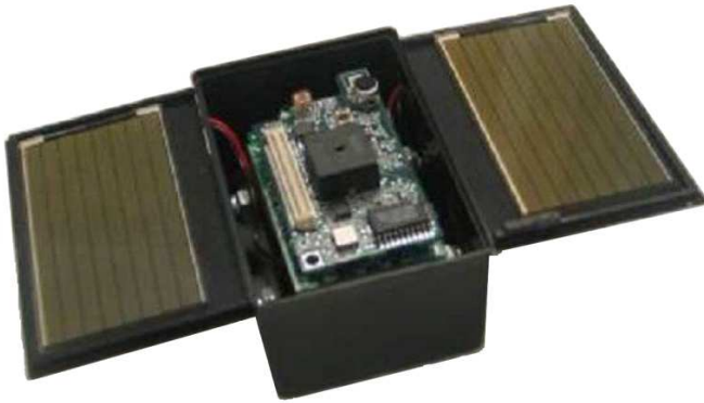
Fig. 3. Heliomote, a solar harvesting sensor node.
