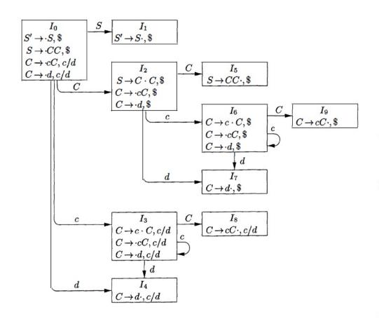
$$\begin{array}{cccc} S' & \to & S \\ S & \to & C C \\ C & \to & c C \mid d \end{array}$$
