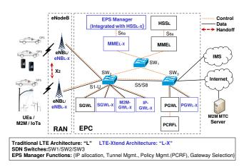
Figure 1: Conventional LTE and LTE-Xtend system architectures. LTE-Xtend components are shown in a different color. L and L-X subscript indicates components for conventional LTE and LTE-Xtend, respectively.
