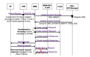
Figure 2: LTE-Xtend M2M/UE attach procedure control flow diagram.
