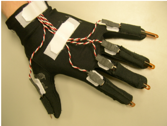
Figure 3. Data glove providing input to FingerSpell.
