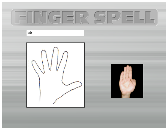
Figure 4. FingerSpell interface shows the word that was just spelled. Open-hand gesture indicates end of a word.
