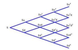
Although there are  $2^n$  distinct paths through this *n*-stage network there are only  $\binom{n}{2}$  nodes, so we can efficiently compute the *exact* distribution of paths through this network!
