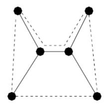
The Option Traveling System tour is at most twice the length of the minimum spanning tree.
