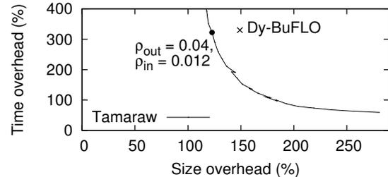
Figure 4: The lower-left boundary of the two-dimensional feasibility region of size and time overhead for Tamaraw when varying  $\rho_{out}$  and  $\rho_{in}$ . Our chosen parameters and the overhead of BuFLO on the same data set are marked. The overhead includes the padding mandated by  $L = 100$ .
