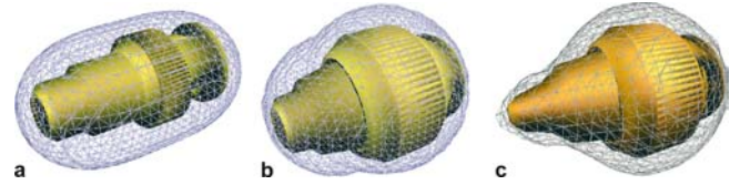
Fig. 7. Mesh-warping of an engineering model
