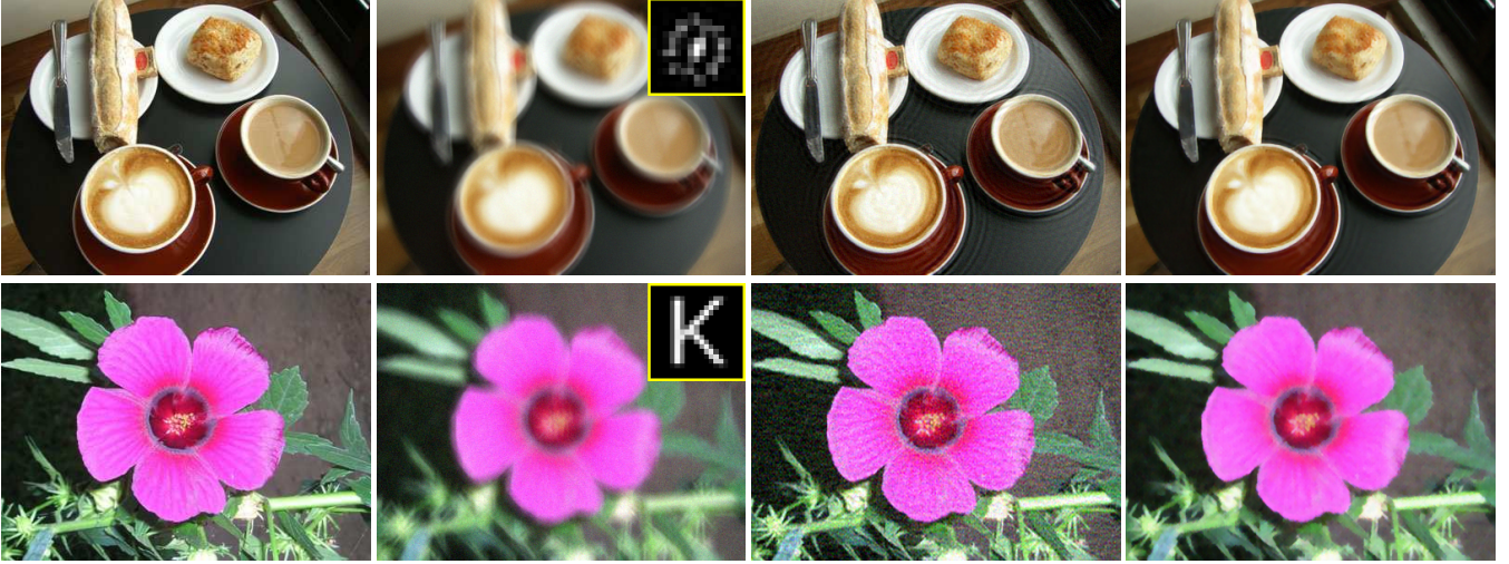
Fig. 3. More deblurring results, from left to right: original images, blurred images with Gaussian noise ( \sigma = 0.03 ), results by sparse prior [2], and our results.
