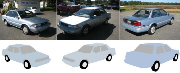
Figure 5. Albedo estimation. The original input images are shown in the first row and estimated albedos are shown in the second row. The two left images come from the same car and the right-most image comes from another car.
