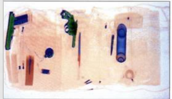
Typical Threat Objects Dual Energy Organic/Inorganic Identification
