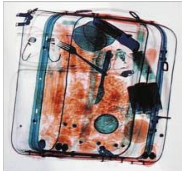
Typical Threat Objects Dual Energy Organic/Inorganic Identification
