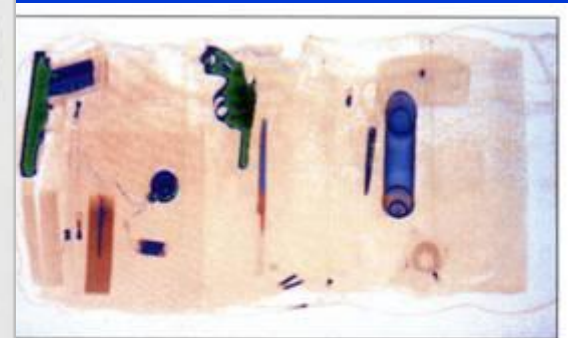
Typical Threat Objects Dual Energy Organic/Inorganic Identification
