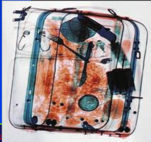
Typical Threat Objects Dual Energy Organic/Inorganic Identification
