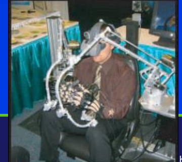
Force feedback exoskeleton Haptic workstation
