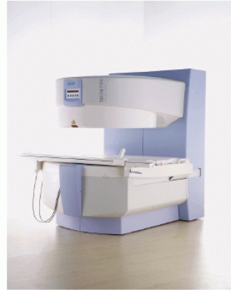
Open (C-shaped) scanner (0.2 T) helps with claustrophobia open space improves patient handling can be used for MRI- guided procedures SNR low and field homogeneity poor
