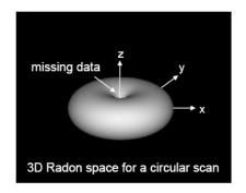
By a circular source trajectory a donut shaped region is acquired in 3D Radon space. At the z-axis a cone-like region is missing.
