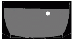
Normal phantom (simulated water with iron rod)
