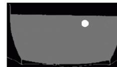
Normal phantom (simulated water with iron rod)
