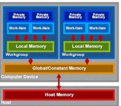
**Execution Model** SPIE Medical Imaging OpenCL CPU GPU Context Programs Kernels Memory Objects **Command Queues** dp\_mul Buffers Images \_\_kernel void dp\_mul(global const float \*a, global const float \*b, global float \*c) dp\_mul CPU program b Out of In arg[0] value Order Order dp\_mul GPU program bir Queue arg[1] value Queue int id = get\_global\_id(0); c[id] = a[id] \* b[id]; arg[2] value GPU Create data & Compile code arguments
