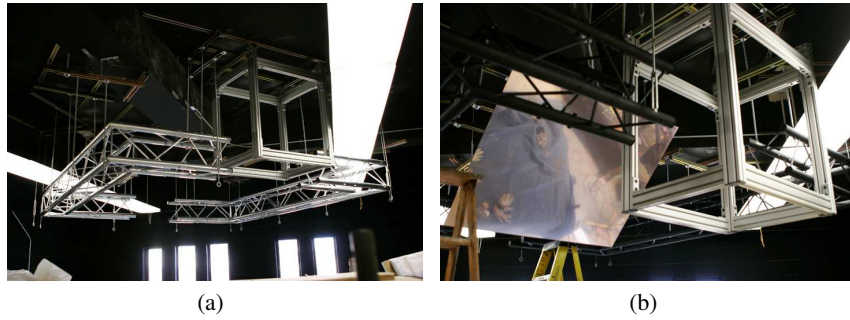
Fig. 4. (a) Screen hanging cables, aluminum trusses mounted to the ceiling, and (b) aluminum trusses painted in black to minimize light reflection and the floor projection mirror
