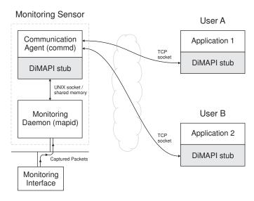
Fig. 3. Architecture of a LOBSTER monitoring sensor.
