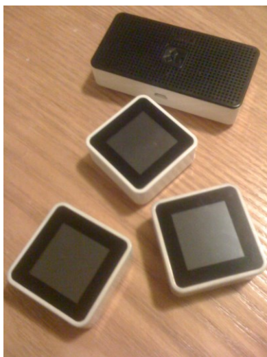
Figure 3. Sifteo Cubes are tangible input/output devices that communicate with a base (located above the three cubes in the picture). Our game, Mind Reader, took advantage of the cubes' LCD screen, touch capability, and small lightweight design.
