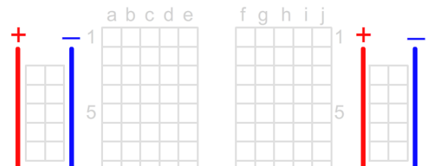
Fig. 2. Power Pin (in both left and right sides) and Regular Pin (in the middle) representation in the presentation layer of the virtual breadboard.
