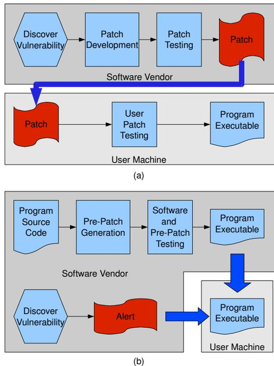
Figure 1: (a) The steps of traditional patch development and deployment. (b) Software development and “patch” deployment with pre-patched software.
