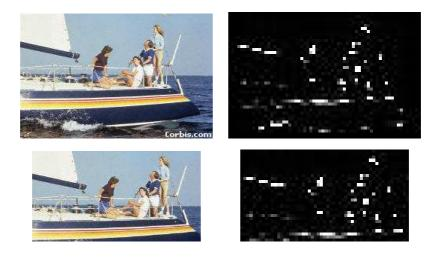
Figure 7.5: (left top): the original image (courtesy of Corbis [3]); (right top): the saliency map; (left bottom): the cropped image; (right bottom): the cropped saliency map which contains most of the salienct parts.
