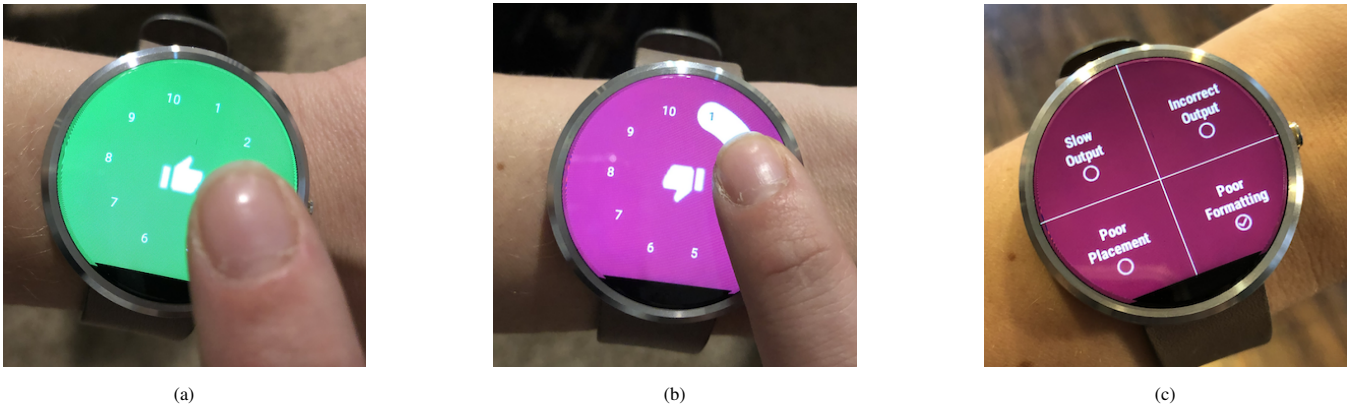
Figure 5: Tester using ARCHIE annotator to provide feedback: (A) tapping to toggle between affirmative and negative reactions, (B) scrolling along the edge of the watch to rate her experience, (C) selecting issues she experienced from a grid of options.
