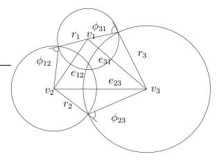
Figure 4: Circle packing metric for a triangle. Triangle  $[v_1, v_2, v_3]$  has vertices  $v_1, v_2, v_3$ , and edges  $e_{12}, e_{23}, e_{31}$ . Three circles centered at  $v_1, v_2$ , and  $v_3$ , with radii  $\gamma_1, \gamma_2$  and  $\gamma_3$  intersect one another, with intersection angles of  $\Phi_{12}, \Phi_{23}$  and  $\Phi_{31}$ , which are the weights associated with the edges. The edge lengths of the triangle are determined by  $\gamma_i$  and  $\Phi_{ij}$  by the cosine law.
