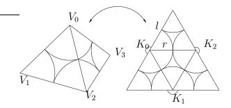
Figure 5: Circle packing metric and curvature. For a canonical tetrahedron, the edges lengths are all l = 1.0, and the radius at each vertex is r = 0.5. The curvature on each vertex equals to  $K_i = \pi$ . The weights on all edges are  $\Phi = 0$ .
