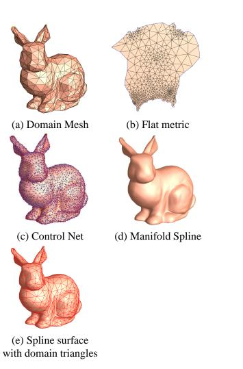
Figure 14: **Manifold spline for an open surface.** The bunny mesh has three boundaries, two are at the ear tips, one is at the bottle. The affine atlas is computed using Ricci Flow under free boundary condition.
