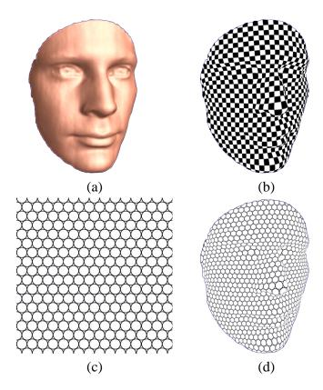
Figure 1: **Conformal mapping and its properties.** Conformal mappings preserves angles, the right angles of checkers in are preserved in (b). Conformal mapping transforms the infinitesimal circles on the texture plane to the infinitesimal circles on the surface, it also preserves the tangency of circles.
