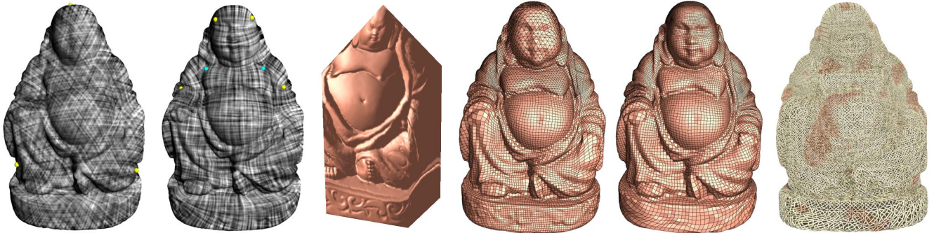
Figure 1: Metric-driven N -RoSy field design. From left to right, a 3-RoSy field, a 4-RoSy field, a flat cone metric visualized as an obelisk, triangle-quad mixed remeshing based on the metric, quad-remeshing, woven Celtic knot design over the surface based on the quad-remeshing.
