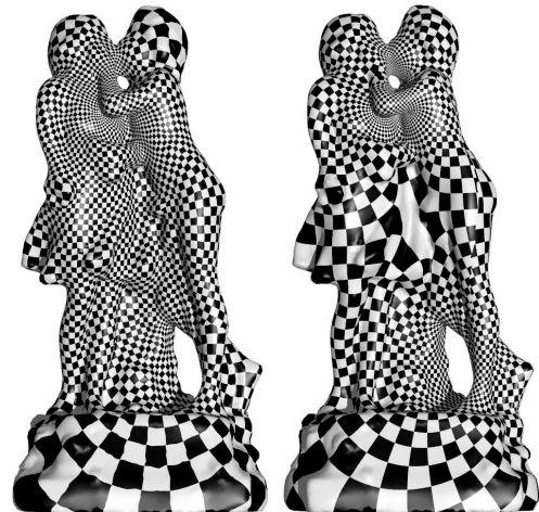
Fig. 12. Euclidean vs. Hyperbolic The right one was conformally parameterized to a Euclidean plane with 4 singularities, while the left one was conformally parameterized to the Poincaré disk and is singularity-free.
