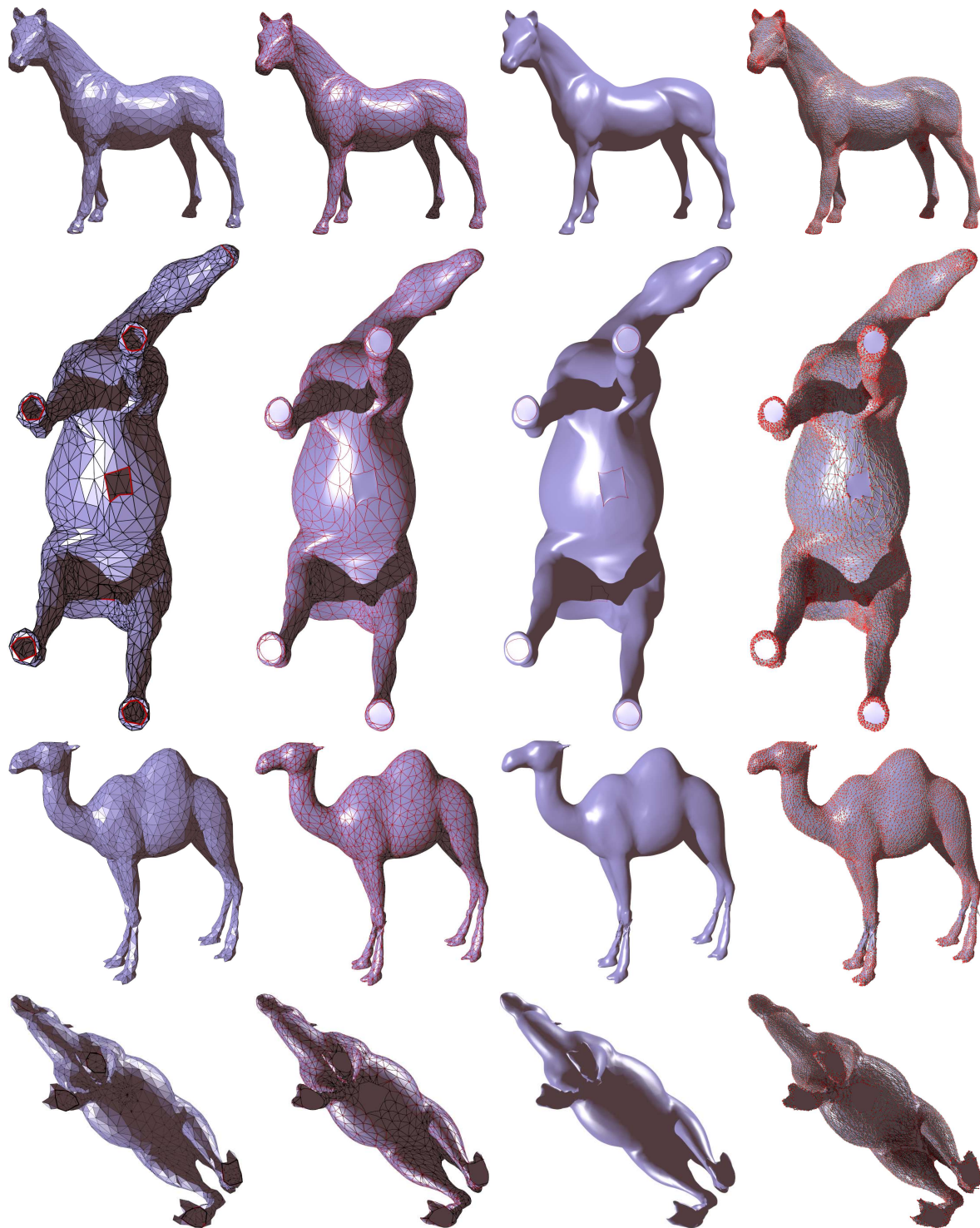
Fig. 17. Multiple singularities. Within our framework, the user can also specify multiple singularities on the models. The horse model has five boundaries (four on the feet and one on the mouth) and two singularities. The camel model has five boundaries and one singularity. The target geodesic curvature of the boundary vertices is zero. The holes and singularities are filled using minimal surfaces.
