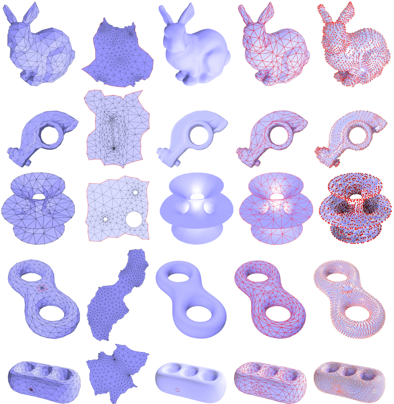
(a) Parametric domain (b) The central chart (c) Manifold splines (d) Spline patchwork (e) Control point distribution
