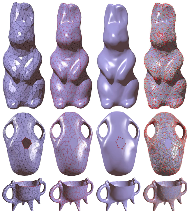
Fig. 14. Examples of manifold splines with various extraordinary points. Rabbit: genus zero, two boundaries, no singularity; Vase: genus two, one singularity; Cup: genus two, one boundary, no singularity.
