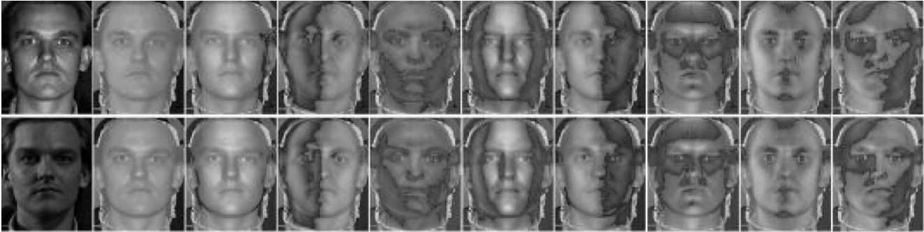
Figure 4. The basis images recovered from an image taken under multiple illuminants (bottom) compared to those recovered from an image under single illumination(top).
