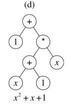
Second offspring of crossover of (a) and (b) picking "+" of parent (a) and left-most "x" of parent (b) as crossover points
