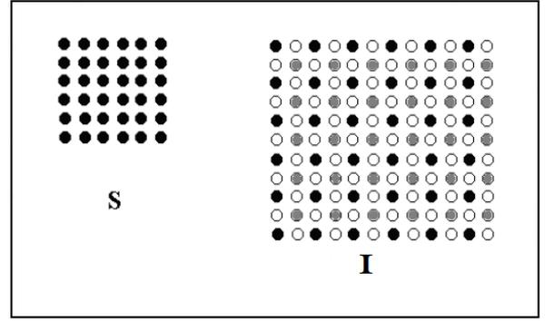
Fig. 1. First stage expansion of an image from Low Resolution to High Resolution (Black dots in image I are original pixels from LR image).
