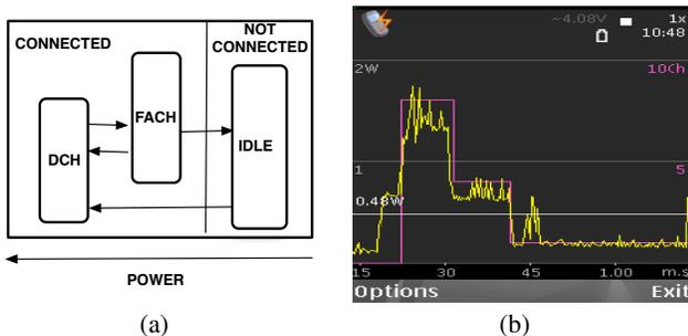
**Figure 1:** (a) The radio resource control state machine for 3GPP networks consisting of three states: IDLE, DCH and FACH (b) Instantaneous power measurements for an example transfer over 3G showing the transition time between high to low power state
