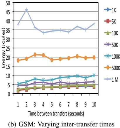
**Figure 6: GSM Measurements:** (a) Average ramp, transfer and tail energy consumed to download 50K data. The lower portion of the stacked columns show the proportion of energy spent for each activity compared to the total energy spent. (b) Average energy consumed for downloading data of different sizes against the inter-transfer time.
