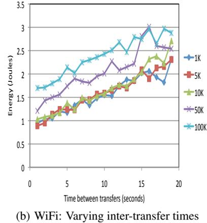
**Figure 7: WiFi Measurements:** (a) Average scan/associate and transfer energy consumed to download 50K data. The lower portion of the stacked columns show the proportion of energy spent for each activity compared to the total energy spent. (b) Average energy consumed for downloading data of different sizes against the inter-transfer time.
