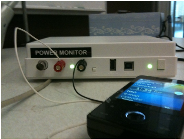
Figure 5: The hardware power meter used for energy measurements.
