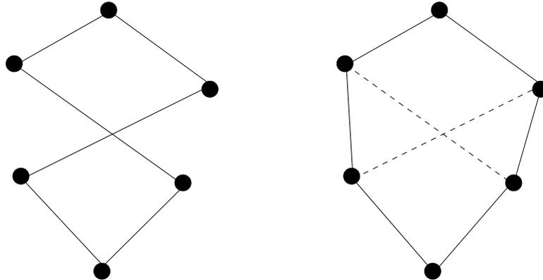
Since only four edges change in the tour, the transitions can be performed and evaluated faster. Faster transitions mean that we can evaluate more positions in the given amount of time.
