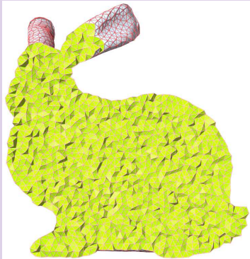
Figure: Volumetric morphing using Levy's method.
