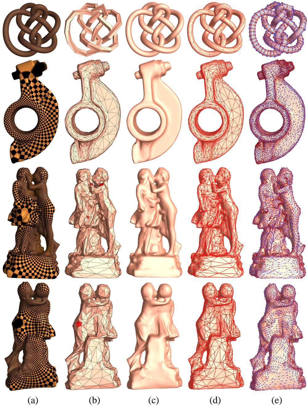
Fig. 11. Manifold spline examples: (a) Holomorphic 1-form \omega which induces the affine atlas \mathcal{A} ; (b) Parametric domain manifold M with singular points Z marked; (c) Polynomial spline F defined on the manifold M in (a); (d) The red curves on spline F correspond to the edges in the domain manifold M ; (e) Spline F covered by control net C .
