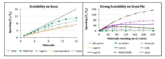
FIGURE 8.5: Strong scalability on Xeon and Xeon Phi.
