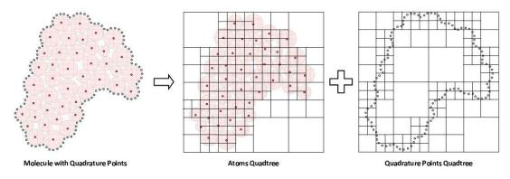
FIGURE 9.1: In the Born radius approximation algorithm two octrees are constructed: one for the atoms in the molecule, and the other for the quadrature points. Born radii of all atoms are approximated by recursively traversing both octrees simultaneously. For simplicity, the octrees are drawn as quadtrees. This figure has been reused from [45] with permission.
