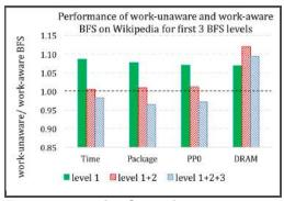
FIGURE 8.6: This figure shows energy consumption by different components of the machine (Package = Socket (CPUs), PP0 = Power Plane0) for the first 3 BFS levels.
