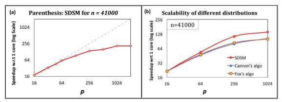
FIGURE 3.20: Parenthesis Problem: (a) Scalability of shared-distributed-sharedmemory algorithm (offloading functions C and B). (b) Performance comparison of different work distribution techniques (offloading C only).
