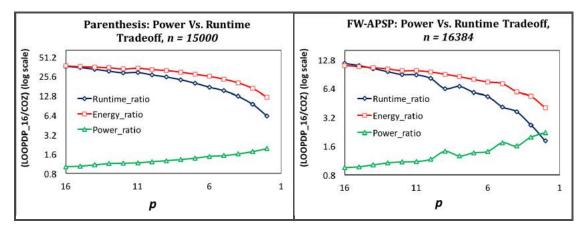
FIGURE 3.16: Power and Runtime Tradeoff. CORDAC has the flexibility to use fewer number of cores while still running faster but consuming less energy and power than LOOPDP.
