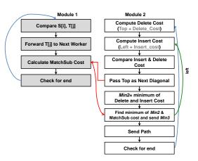
FIGURE 2.7: Flow chart for the control flow path of a single worker. Blue arrows show state transitions, green arrows show self-feedback, and red arrows show communication with other PEs.
