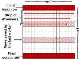
FIGURE 2.9: Strip mining using standard memory and scratchpad memory. Initial and final rows are read from and written to memory, while the intermediate rows use either memory or scratchpad memory.
