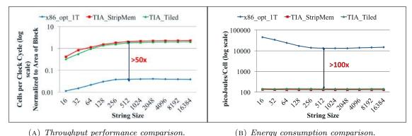
FIGURE 2.13: Results showing that implementations on triggered instruction spatial architecture (TIA) run  $50 \times$  faster while consuming  $1/100 \times$  energy compared to the optimized single-threaded x86 based tiled-loop implementation.
