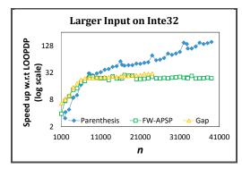
FIGURE 3.14: Speedup w.r.t LOOPDP with larger input sizes on Intel32 machine.
