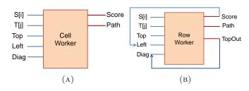
FIGURE 2.5: (A) A simple cell worker that computes a single cell of the cost matrix, (B) An optimized row worker.
