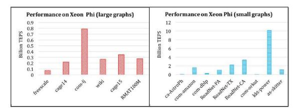
FIGURE 8.4: Performance on Xeon Phi (manycores).
