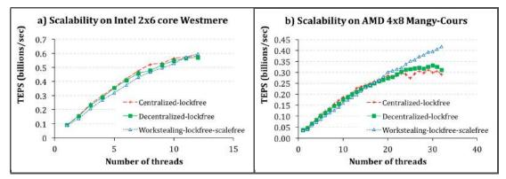
FIGURE 7.1: Scalability of lockfree parallel BFS algorithms running on (a) Lonestar and (b) Trestles. All algorithms were run on the Wikipedia graph. All programs were implemented using Intel<sup>®</sup> Cilk++™.
