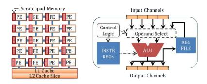
FIGURE 2.2: Example spatial architecture. Network of PEs, scratchpad memory, and caches are shown alongside a PE diagram.
