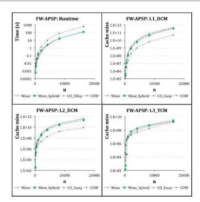
FIGURE 5.4: Runtime and cache misses in three levels of caches for 2-way CO (COR-DAC), COW and recursive wavefront algorithms for the 2D FW-APSP Problem. All programs were run on 16 core machines in Stampede. All implementations used Cilk Plus's work-stealing scheduler.
