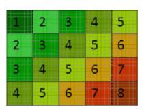
FIGURE 2.12: Execution pattern of the x86 based tiled-loop code. The numbers on the tile shows when a tile get executed. Tiles with the same numbers gets executed in parallel.
