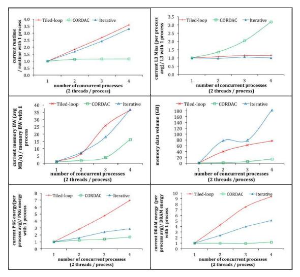
FIGURE 4.4: The plots show how the performances of standard-iterative, tiled-loop and recursive codes for solving the Floyd-Warshall APSP problem (for  $n = 2^{12}$ ) are affected as multiple instances of the same program are run on an 8-core Intel Sandy Bridge processor with 20MB shared L3 cache.
