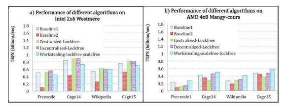
FIGURE 7.2: Performance in terms of Traversed Edges Per Second (TEPS) when traversing real-word graphs on machines from (a) Lonestar (12 cores) and (b) Trestles (32 cores). All programs were implemented using Intel<sup>®</sup> Cilk++<sup>™</sup>.
