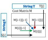
FIGURE 2.4: Data flow dependencies for calculating a cell in edit distance. Dependencies are found along the row and column of the cost matrix, which limits the ability to vectorize.
