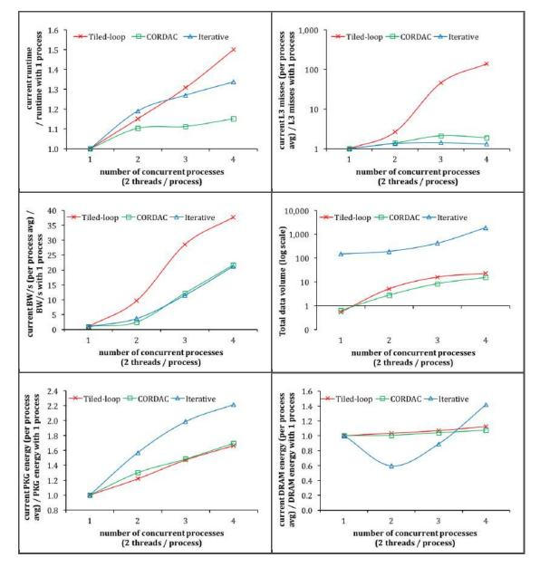
FIGURE 4.5: The plots show how the performances of standard iterative, tiled-loop and recursive codes for solving the Gap problem (for  $n = 2^{13}$ ) are affected as multiple instances of the same program are run on an 8-core Intel Sandy Bridge processor with 20MB shared L3 cache.
