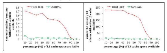
FIGURE 4.6: The plots show how changes in the available shared L3 cache space affect the serial running time and the number of L3 cache misses of tiled-loop and recursive (CORDAC) algorithms for solving the parenthesis problem when  $n = 2^{13}$ . The code under test was run on a single core of an 8-core Intel Sandy Bridge processor with 20MB shared L3 cache. A multithreaded Cache Pirate [1, 70] was run on the remaining 7 cores to steal L3 cache space.
