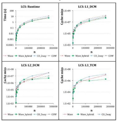
FIGURE 5.3: Runtime and cache misses in three levels of caches for 2-way CO (COR-DAC), COW and recursive wavefront algorithms for the LCS Problem. All programs were run on 16 core machines in Stampede. All implementations used Cilk Plus's workstealing scheduler.
