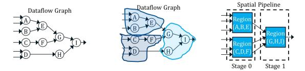
FIGURE 2.1: Spatial programming example. Converting a dataflow graph to a spatial pipeline of regions.
