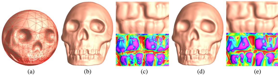
Figure 5: Illustration of our fairing algorithm for a spherical triangular  $B$ -spline: (a) A degree 5 spline with 948 patches. (b) The mean curvature of (a) (red,  $H < 0$ , cyan,  $H > 0$ , green,  $H \approx 0$ ). Pay attention to the high curvature concentration along the image of edges of the spherical triangles. (d)-(e), After fairing, the curvature distribution improves significantly.
