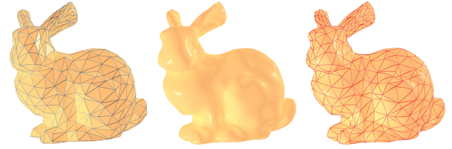
Fig. 5: Interpolatory spline on the Bunny model with |V| = 500 vertices. The biharmonic B-spline f(x) interpolates all vertices, f(v_i) = v_i, i = 1, \dots, |V| . The red curves are the images of the edges of M .
