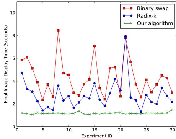
**Figure 4.** Final image display time of binary swap, radix-k, and our algorithm.  $N = 32$ , computing power range =  $(1, 10^3)$ , link bandwidth range =  $(1, 10^2)$ , and link latency range =  $(10^{-5}, 10^{-3})$ . Radix-k uses the configuration [4, 4, 2].
