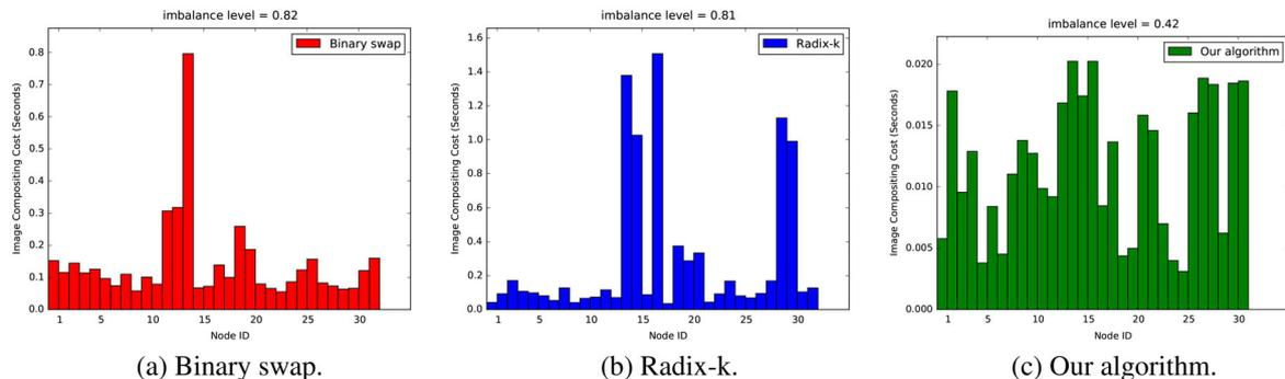
**Figure 5.** Load-balancing results of binary swap, radix-k, and our algorithm.  $N = 32$ , computing power range =  $(1, 10^3)$ , link bandwidth range =  $(1, 10^2)$ , and link latency range =  $(10^{-5}, 10^{-3})$ .
