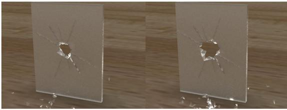
**Fig. 9** A ball collapses through glass window, breaks into a hole and crack propagates without destroying the global structure. Fracture surface normal is the same while different ball sizes lead to different radii. The radii of balls are 3 and 5
