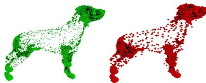
**Fig. 6** Boundary particle generation for a pet model. All the surface particles are used to create the boundary particles with a sampling size. *Left* The original surface particles add up to 11228. *Right* 3678 boundary particles for collision detection
