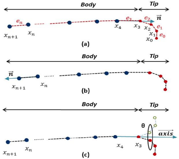
Figure 4. Illustration of different chain-mail constraints corresponding to the pushing, pulling, and rotating operations. In (a) and (b), the blue arrow means the direction of the translation. In (c), the blue arrow is the rotation axis and  $\theta$  means the rotation angle.
