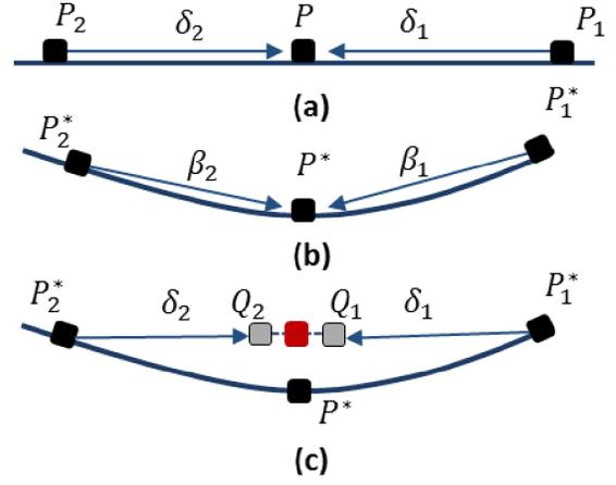
Figure 5. Illustration of physical optimization. From top to bottom: initial shape, deformed shape, optimized shape of the three guidewire chain-mails.
