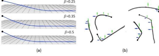
Figure 6. Heterogeneous guidewire simulation results. (a) From top to bottom, the shearing parameters are respectively set to 0.25, 0.35, 0.5, with the same compressing and stretching parameters. (b) The guidewire deformation results obtained by manipulating its soft tip with pulling, pushing, and twisting operations.
