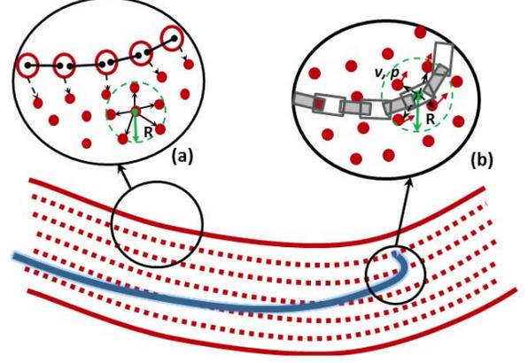
Figure 7. Illustration of heterogeneous chain-mails based coupling model. (a) vessel-blood coupling model. Red circles connected by black lines represent the vascular chain-mail model. Red points connected by green arrows represent the blood-field chain-mail model. The black-dotted lines are the virtual vessel-blood links. (b) guidewire-blood coupling model. Conjoint rectangles represent the guidewire chain-mails. Black-dotted lines are the virtual guidewire-blood links.
