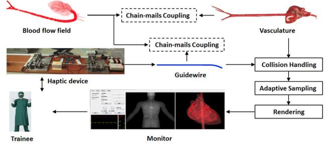
Figure 13. The workflow of guidewire manipulation and simulation in PCI simulator.
