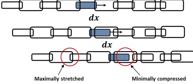
Figure 2. The fundamental principle of the basic chain-mail model. The black arrow means the moving vector of the "sponsoring" element, represented by the blue-filled rectangle. When the distance of adjacent neighbors is less than the minimal compression or larger than the maximal stretch, elements adjust to satisfy the constraint, indicated with the red circle.
