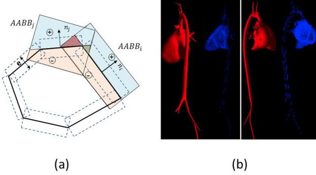
Figure 8. Illustration of collision handling. The Black polygon in (a) represents the vessel,  $\vec{n}$  means the surface normal, dotted boxes are prisms of vascular mesh and solid-line boxes are AABB of dotted boxes, wherein different colors mean different SDF sign. (b) shows the heart and its SDF.
