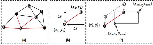
Figure 3. Illustration of the chain-mail updating rule. (a) An arbitrary chain-mail arrangement. (b) The initial state of the "sponsoring" element A and the "affected" neighbor element C. (c) When A moves, C should move to the nearest point within the valid region.
