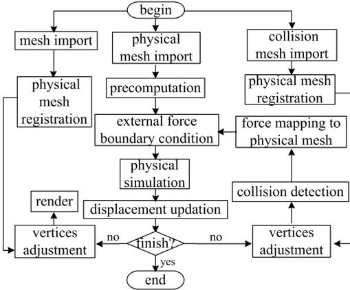
**Figure 3:** The flowchart of the percutaneous coronary intervention simulation system.
