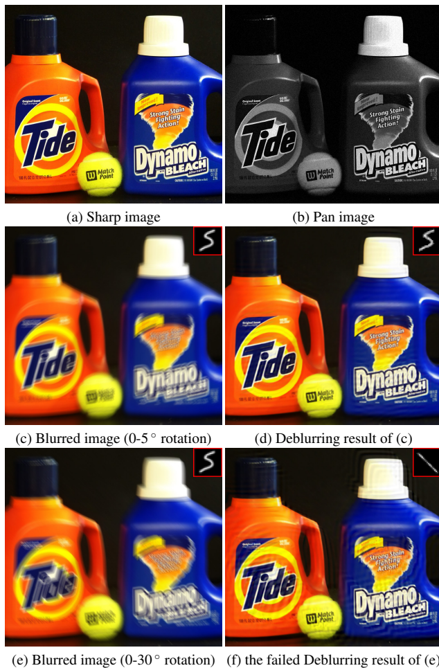
Fig. 11. Examples of spatially variant kernels. We rotate the ground truth kernel in the third dimension from 0^\circ at the top to d^\circ at the bottom of a sharp image (a) to synthesize blurred images (c) and (e) with non-uniform blurs. The deblurring results are shown in (d) and (f), respectively. For a large spatially variant blur in (e), our deblurring result (f) has failed.
