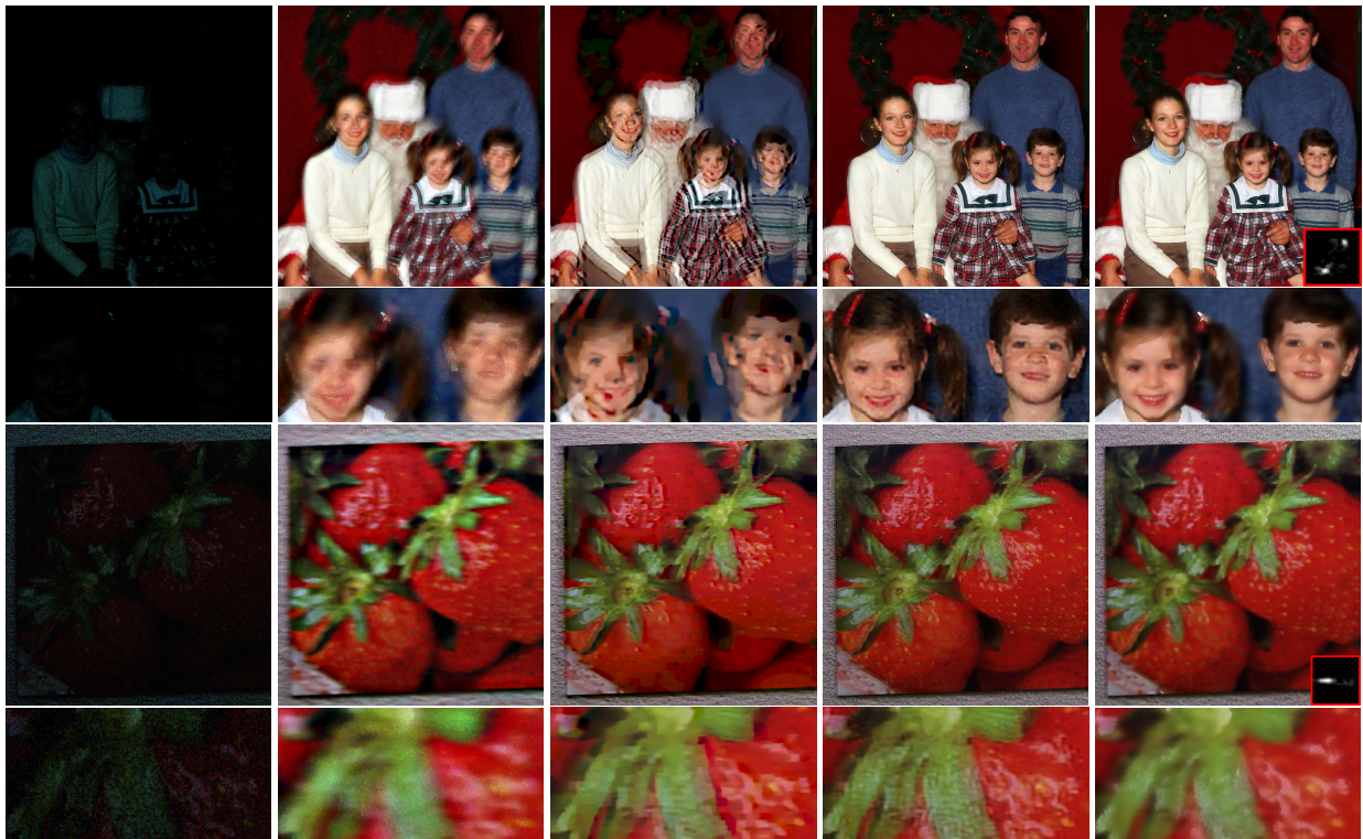
Fig. 8. Experiments on large noise. From Left to Right: noisy images, [Yuan et al. 2007], [Cho and Lee 2009], [Xu and Jia 2010], and our method.
