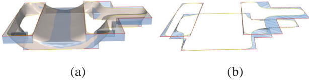
Fig. 6. Constructing the mapping between boundary curves \partial P_i to \partial M_i . (a) The boundaries of P_i and M_i are planar curves. (b) The blue lines show the map \psi_i between the vertices on \partial P_i and \partial M_i (see Equation 6).
